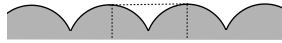
Fig. 2 A simple billiard microstructure consisting of arcs of circle. We refer to it as the bumps family . The (scale-invariant) curvature of the bumps is defined by K = L/R , where L is the distance between two consecutive corner points and R is the radius of the circular arcs. We assume throughout, without loss of generality, that L = 1 . This paper is concerned with properties of this particular family, as a function of K , for small values of K . A billiard cell is indicated by the dashed lines
